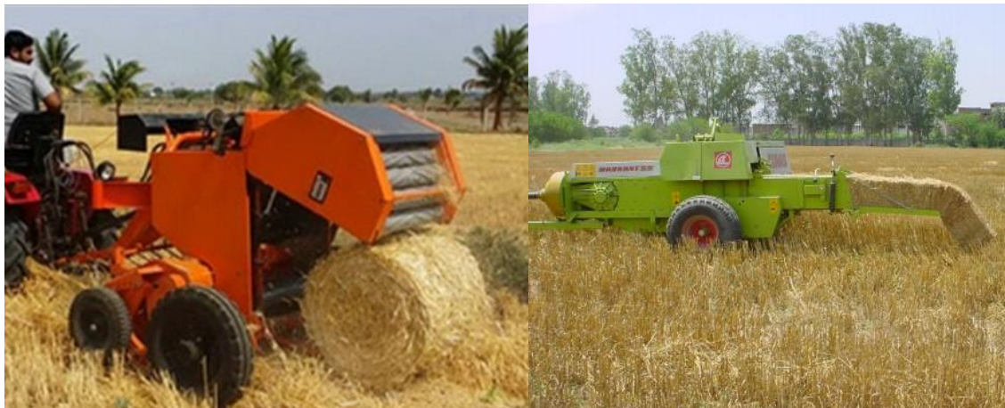
Fig 4 Mechanized paddy straw collection with a tractor drawn round and square baler From harvest paddy field
