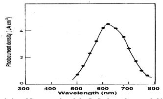
Fig: 18. – Variation of J<sub>ph</sub> vs wavelength for In<sub>2</sub>S<sub>3</sub> electrodes annealed in argon at 500°C
