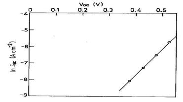
Fig: 14. – In J<sub>sc</sub> Vs V<sub>oc</sub> plot for In<sub>2</sub>S<sub>3</sub> films deposited at 50 % duty cycle
