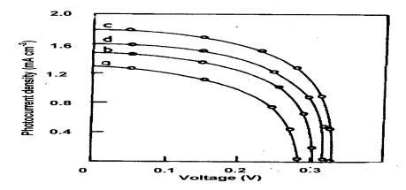
Fig: 9. – Load characteristics of In<sub>2</sub>S<sub>3</sub> films deposited at 6 % duty cycles and post heat treated at different temperatures (a) 400°C (b) 450°C (c) 500°C and (d) 525°C
