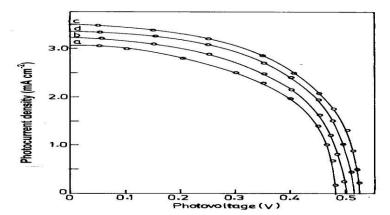
Fig: 13. – Load characteristics of In<sub>2</sub>S<sub>3</sub> films deposited at 50 % duty cycles and post heat treated at different temperatures (a) 400°C (b) 450°C (c) 500°C and (d) 525°C
