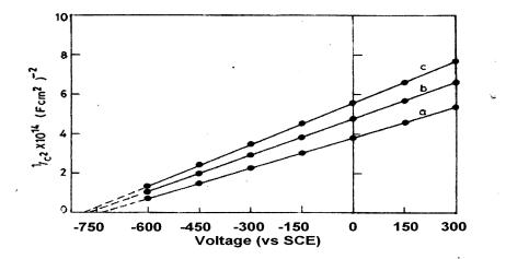
Fig: 17. – Mott Schottky plots of  $In_2S_3$  electrodes annealed in argon at different temperatures (a) 450°C (b) 500°C (c) 550°C
