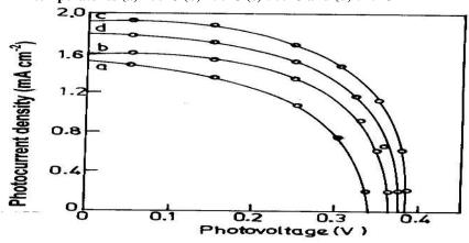
Fig: 10. – Load characteristics of In<sub>2</sub>S<sub>3</sub> films deposited at 9 % duty cycles and post heat treated at different temperatures (a) 400°C (b) 450°C (c) 500°C and (d) 525°C
