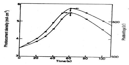
Fig: 15. – Variation of Photocurrent and photovoltage with photoetching time of 60 s, In<sub>2</sub>S<sub>3</sub> photoelectrodes deposited at 50 % duty cycle and post heated at 500°C
