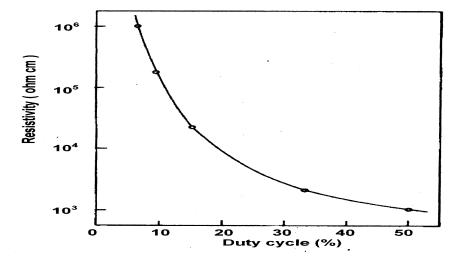
Fig: 8. – Variation of resistivity with duty cycle for In<sub>2</sub>S<sub>3</sub> films
