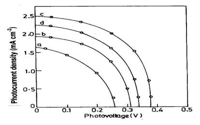
Fig: 12. – Load characteristics of In<sub>2</sub>S<sub>3</sub> films deposited at 33 % duty cycles and post heat treated at different temperatures (a) 400°C (b) 450°C (c) 500°C and (d) 525°C
