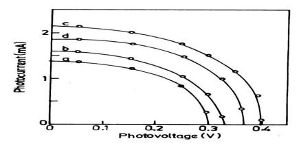
Fig: 11. – Load characteristics of  $In_2S_3$  films deposited at 15 % duty cycles and post heat treated at different temperatures (a)  $400^{\circ}C$  (b)  $450^{\circ}C$  (c)  $500^{\circ}C$  and (d)  $525^{\circ}C$
