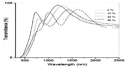
Fig: 6. – Transmission spectra of In<sub>2</sub>S<sub>3</sub> films deposited at different duty cycles
