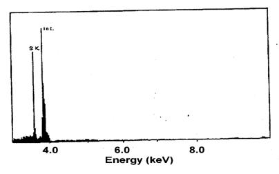
Fig: 2. – EDAX spectrum of In<sub>2</sub>S<sub>3</sub> films deposited at 50 % duty cycle
