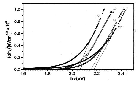
Fig: 7. –  $(\alpha hv)^2$  versus hy plot of In<sub>2</sub>S<sub>3</sub> films deposited at different duty cycles (a) 50 % (b) 33 % (c) 15 % (d) 6 %
