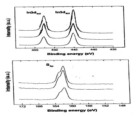
Fig: 3. – XPS spectra of In and S for  $In_2S_3$  films deposited at different duty cycles (a) 15 % (b) 33 % (c) 50% (Bottom to top)
