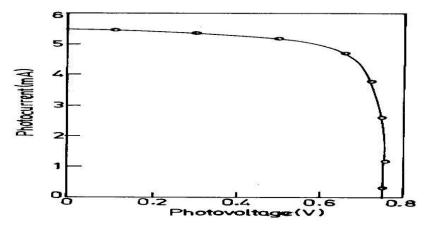
Fig: 16. – Load characteristics of  $In_2S_3$  photoelectrodes deposited at 50 % duty cycle and post heat treated at 500°C after photoetching for 60s.
