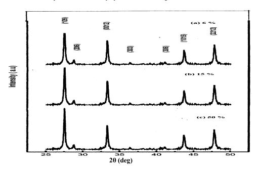
Fig: 1. - X-Ray diffraction pattern of In<sub>2</sub>S<sub>3</sub> films deposited at different duty cycles
