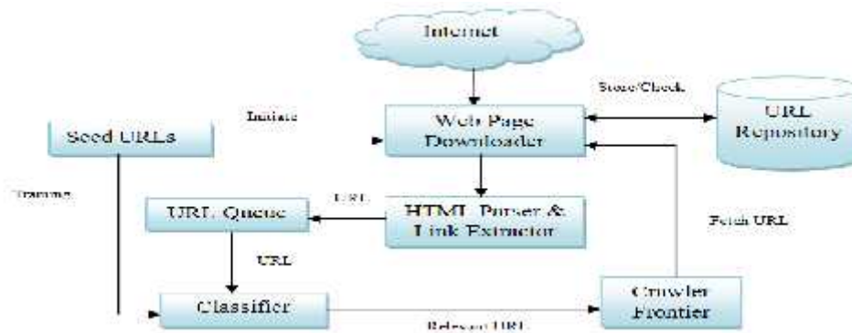
Figure 5: System Architecture of Focused Web Crawler
