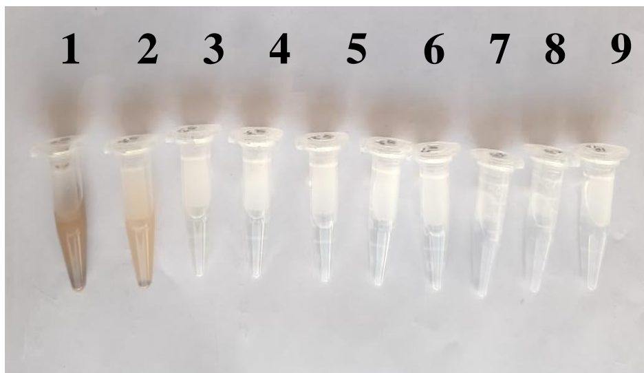
Figure no. 1: Serial dilution of soil sample for the isolation of soil microbes
