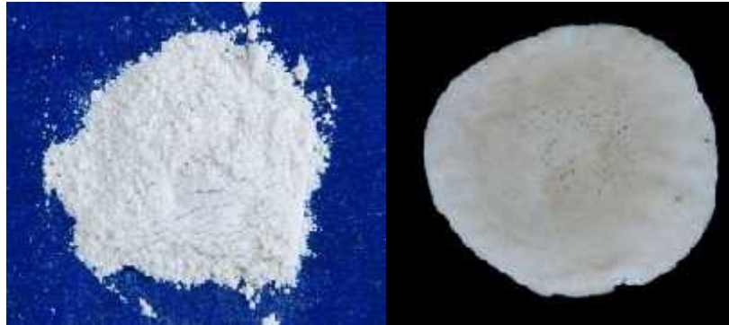
Fig.4. Photographs of \text{CeZrO}_{3.5} nanopowder and \text{CeZrO}_{3.5}/\text{PMMA} nanocomposite
